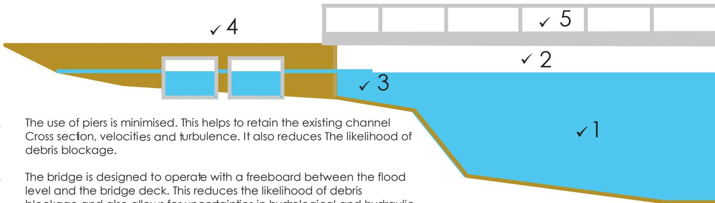
1. The use of piers is minimised. This helps to retain the existing channel Cross section, velocities and turbulence. It also reduces The likelihood of debris blockage.
