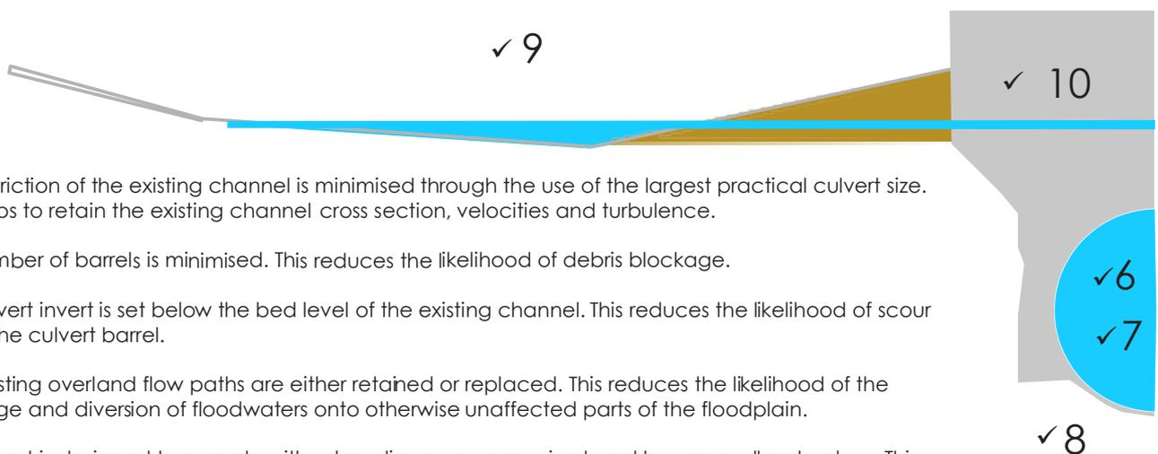
6. The restriction of the existing channel is minimised through the use of the largest practical culvert size. This helps to retain the existing channel cross section, velocities and turbulence.
